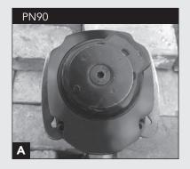
The PN90 model comes with an adjustable exhaust system, loosen the cap bolt as shown, place exhaust in desired direction and re-tighten (clockwise).
